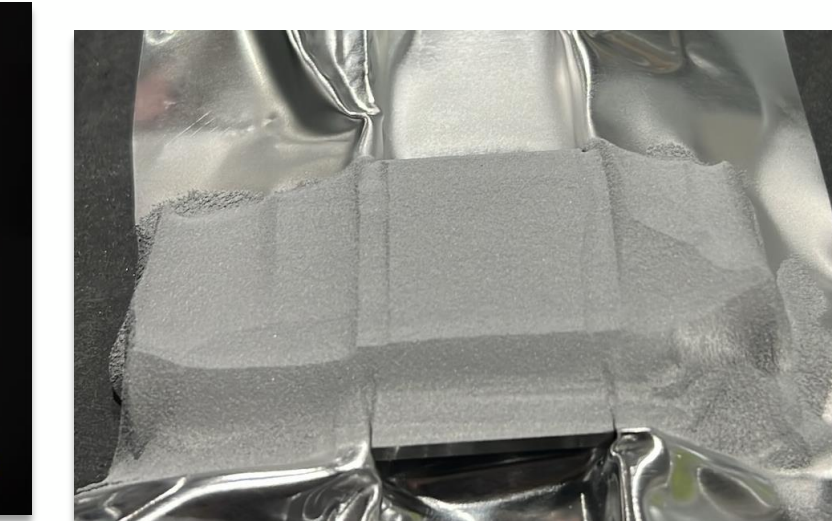
Lug shear sample of Al 6061 deposited onto SMA NiTi substrate.
